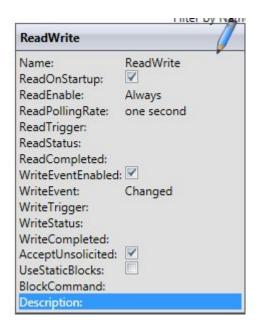
For reading-type points, used as analog measures (Using Get analog changes by sampling mode)
