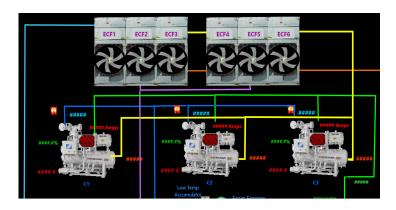
The project used six FactoryStudio Smart (Thin) Clients and 1500 external I/O points. The other system feature that helped Wolverine manage their processes was the ability of FactoryStudio to run in a Virtual Machine with Windows 10 on the Data Center server.
